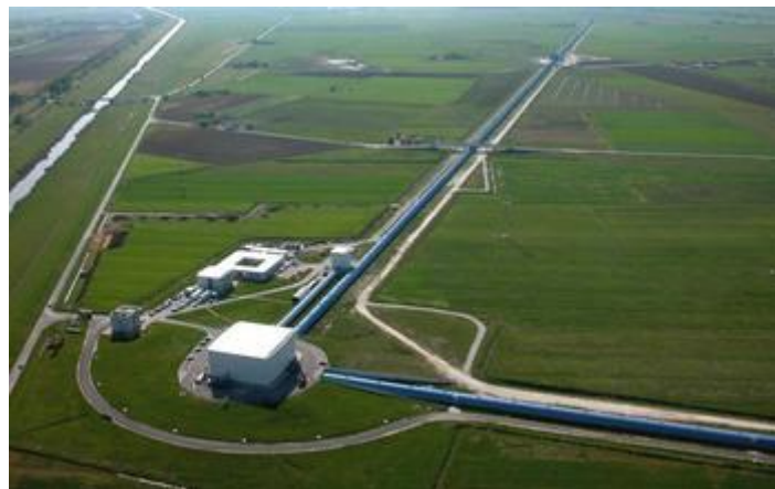
Aerial view of the Virgo site, including the two perpendicular arms of its interferometer. Credit and Larger Version.
