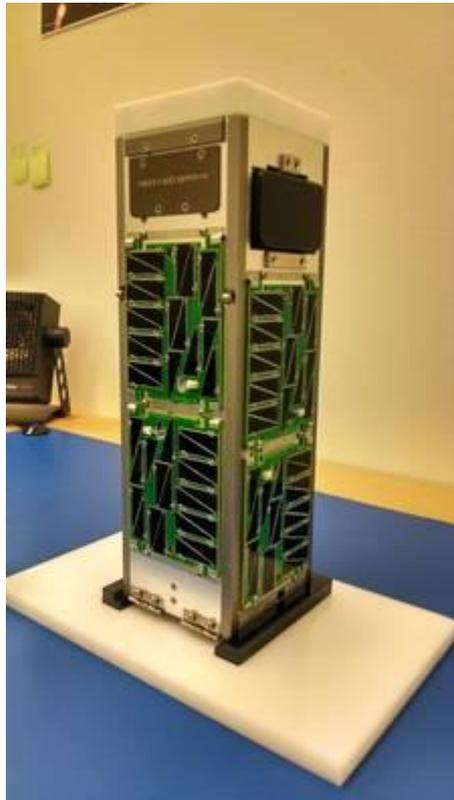
*The TechEdSat series, a technology education collaboration with San Jose State University and the University of Idaho, uses the standard CubeSat structure, which measures one unit (1U) as approximately four inches cubed (10 centimetres cubed). TechEdSat-4 is a 3U satellite. Image Credit: NASA Ames*
