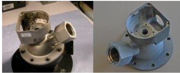
Original and 3D-printed 'woov' valve
