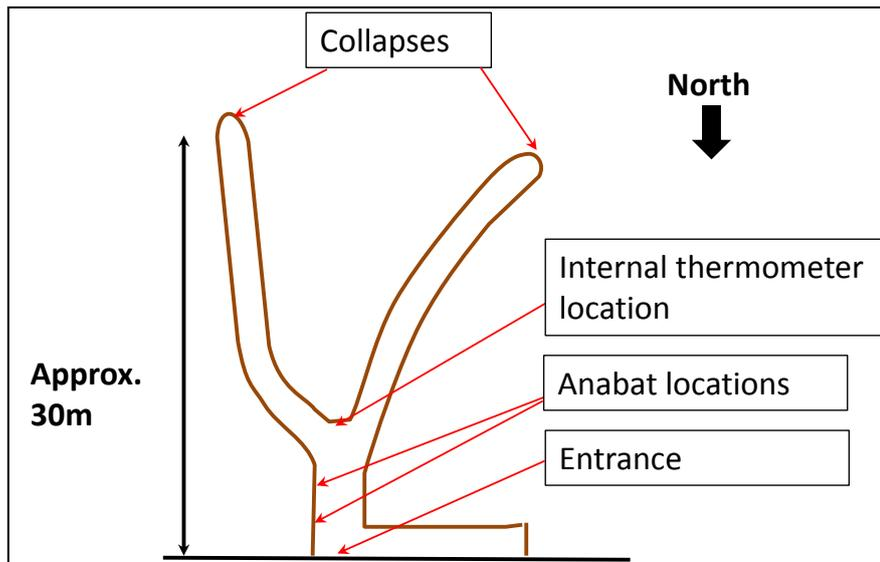
**Image 2** Drawing shows an approximate aerial plan of the currently accessible section of the mine. The mine drops in height several meters from the entrance towards the southern end.
