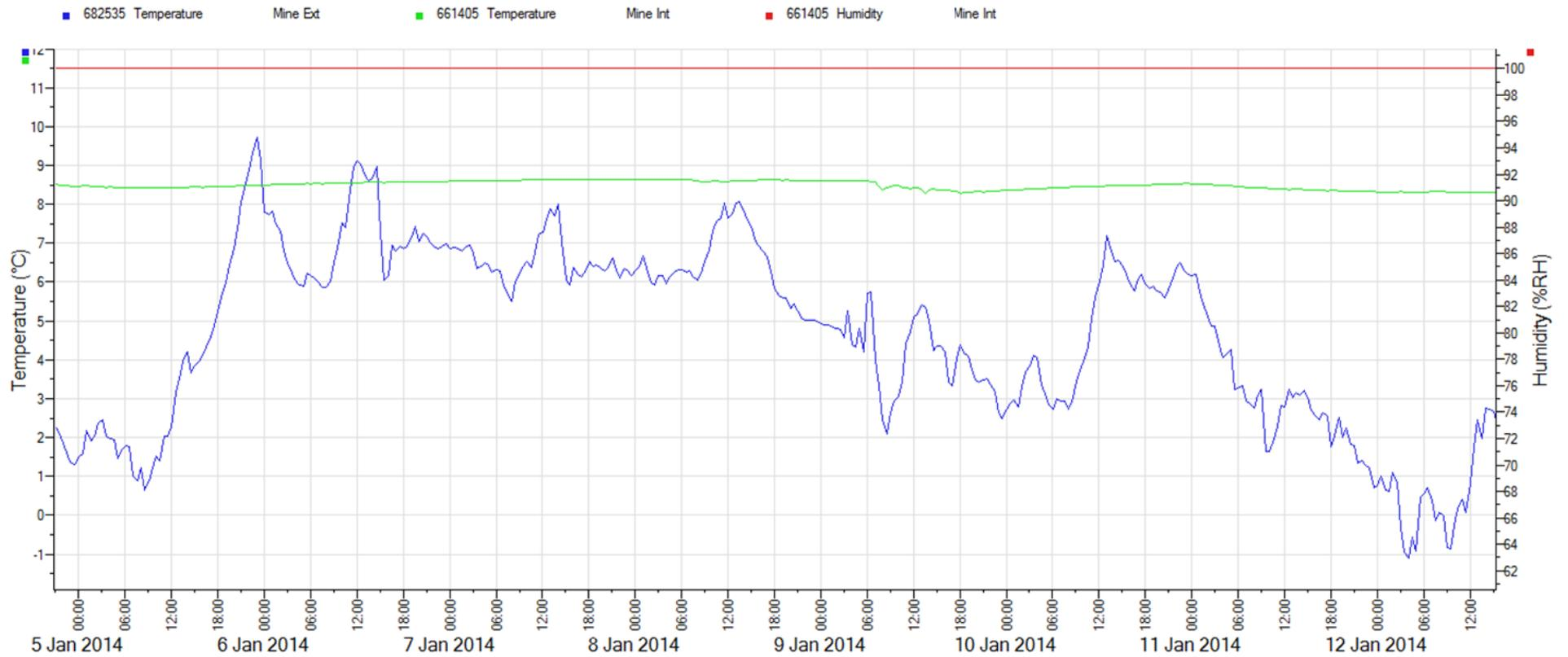
**Figure 3 Comparison of temperature inside (green line) and outside the mine (blue line), with relative humidity inside the mine (red line).**
